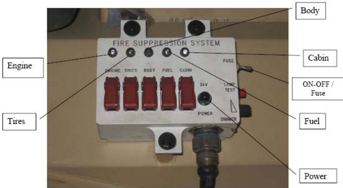
Operation Panel for Fire Suppression System
