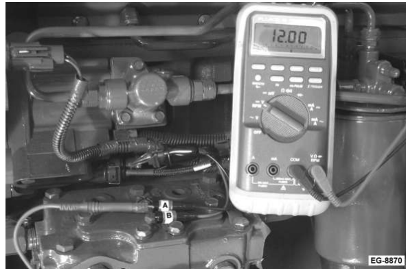
Battery Voltage Measurement
