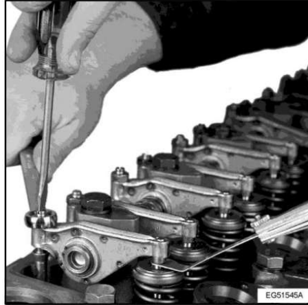
Valve Lash Adjustment
